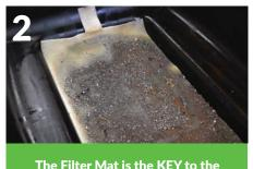
The Filter Mat is the KEY to the system – it contains 200 million oileating microbes and traps particles down to 50 micron.
