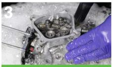
Heated to 42°C, the microbes become active in the ROwash Degreasing solution and eat the oil and grease turning them into harmless CO<sup>2</sup> and water – effectively recycling the fluid.
